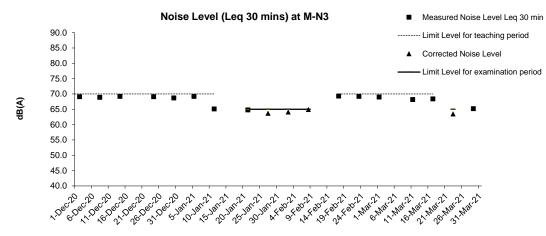
Remark: Corrected Noise Level was applied on 27 January 2021, 2 and 8 February 2021, 23 March 2021; Corrected Noise Level = Measured Noise Level - Baseline Noise Level (i.e. 67.7 dB(A))
